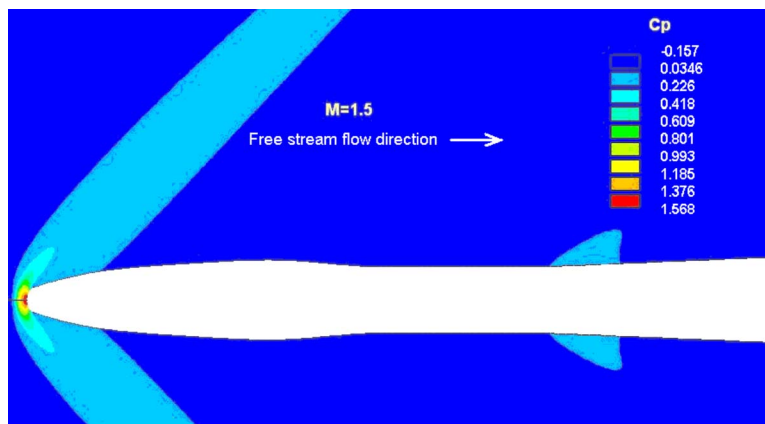
Fig. 5 Supersonic C_p variation near the compensation region of the Pitot tube
